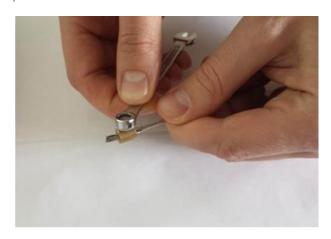
1. Before cable guide installation put sleeves on the cable guides
