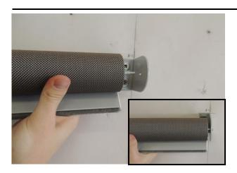
6. Slide the roller tube to bracket from the side opposite the motor by gently pressing the roller tube pin. Then slide the roller tube to the bracket on motor side.
